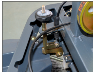
Easy access to broom adjustment system
