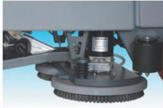
Brush release by foot. No tools required.
